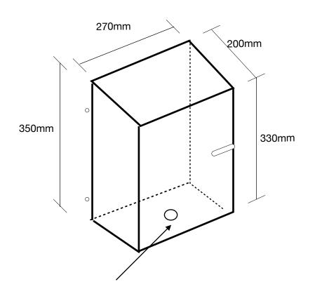
25mm Hole with rubber grommet Set at 80mm centre from the front of the box.
